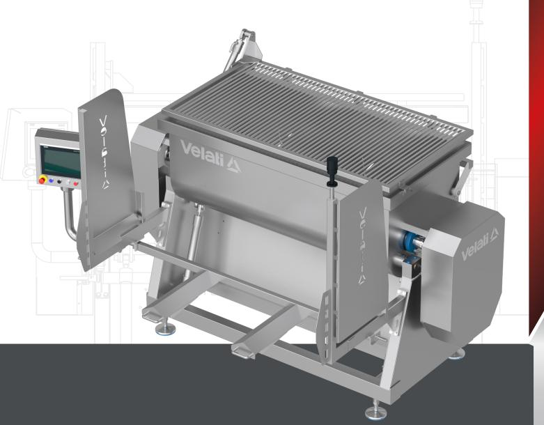
Velati tilting tank mixers – entirely made in stainless steel and with materials suitable for contact with foodstuffs, pursuant MOCA regulations and Hygienic Design principles – are designed for the production of quality cured products, particularly sausages, salami and mortadella.
