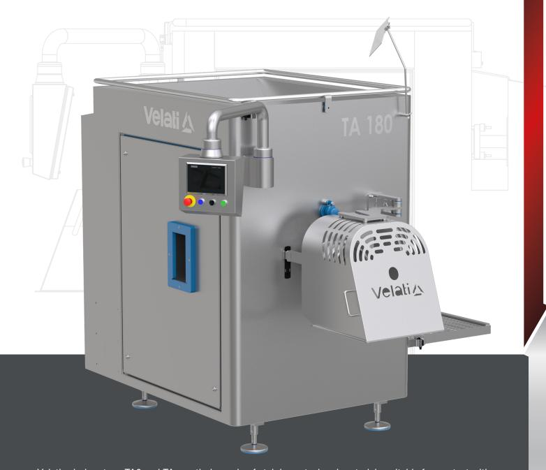
Velati grinders type TA6 and TA – entirely made of stainless steel and materials suitable for contact with foodstuffs, pursuant to MOCA regulations and Hygienic Design – have been designed to process fresh, chilled and frozen meat for small, medium industry, maintaining the same processing characteristics of raw materials.
